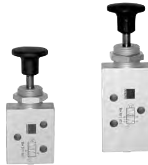
Example: 3/2 and 5/2 manually actuated spool valve, G 1/4", spring return or indexed
